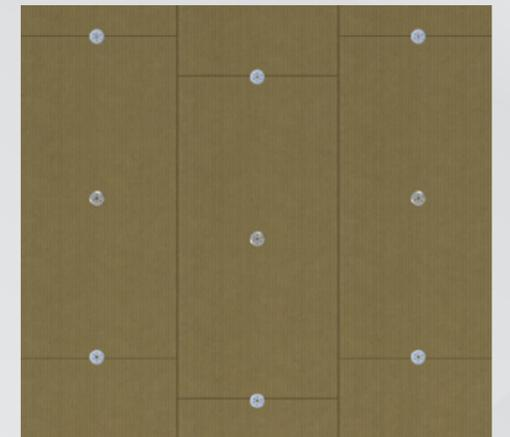
All penetrations, through the insulation layer, at floor junctions and openings should be accounted for in the thermal calculations. For advice on rainscreen fixings, contact the system specifier, ensuring all fixings are accounted for when modelling thermal performance. Guidelines given in BR443 Conventions for U-Value calculations and ISO 6946:2017 Building components and building elements\_\_\_Thermal resistance and thermal transmittance\_\_\_Calculation method should be followed.
